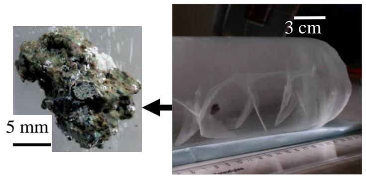
Inclusions are soft aggregates consisting mainly of clay-mica minerals and quartz clasts
