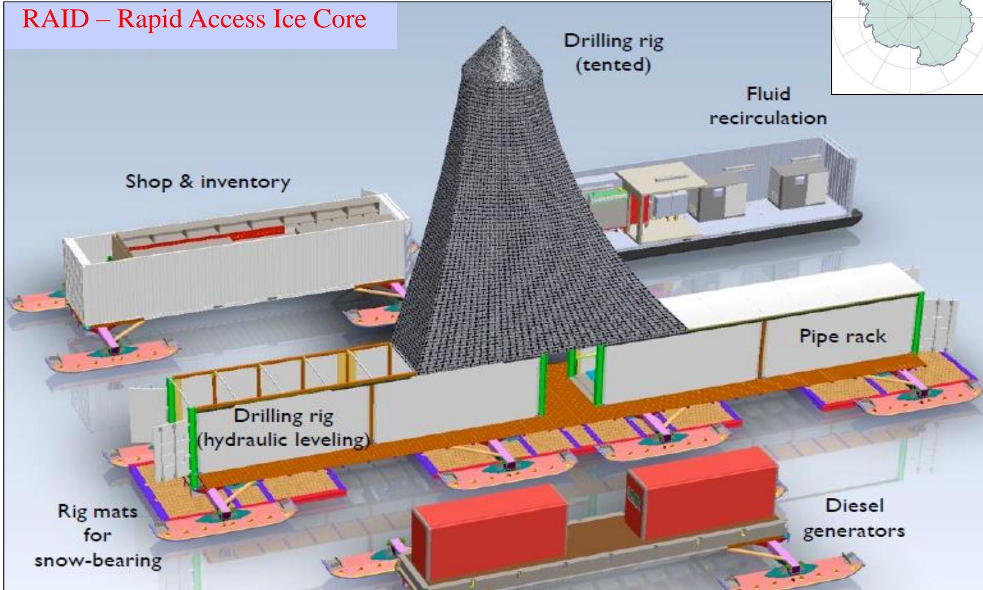
**RAID is designed to penetrate up to 3,3 km of ice 1 week**
