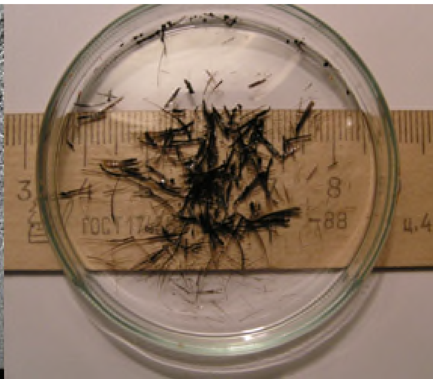
Gel dried: Chains of diamond nanoparticles (TEM, left) Needle-like structures (right)
